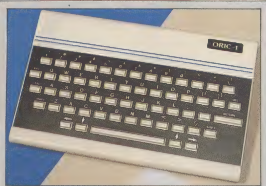
Oric-1 The Atmos is an updated version of the Oric-1. It uses the same circuit board but has a different ROM chip that holds an improved version of BASIC. These changes are sufficient to make the Atmos a far better machine. Owners of the Oric-1 can pay £60 to upgrade to the Atmos standard. However, much of the Oric's software will not work on the Atmos, so users may find themselves unable to use their favourite programs
